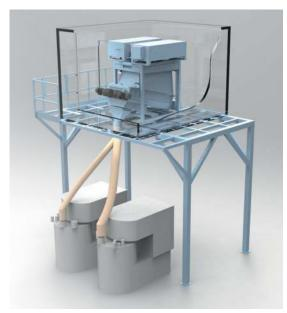
Example of installation: Ice dosage system VS07 with 2 RVH 3000
