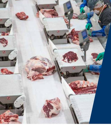
"We have seen that a traditional pace line system takes approximately 20% more people to work it. The StreamLine system is very labor efficient, and more ergonomic as well. The operators do not need to reach for the products – they are led directly to their cutting stations."
