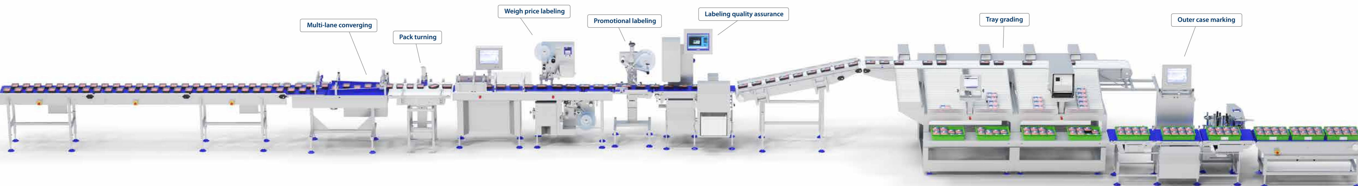
Highly efficient weigh price labeling with automated labeling quality assurance and pack handling
