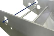
A "line bored" machine cabinet assures perfect alignment between the tooth roll and skinning mechanism that will remain perfectly aligned.
