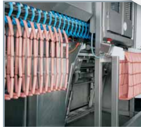
Sausage-making with the iLinker and iConveyor; the RevoPortioner.
