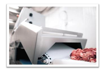
Marel's new trim management system analyses the fat/lean ratio of meat using the X-ray technology of the SensorX, previously used so successfully to detect bones in poultry
