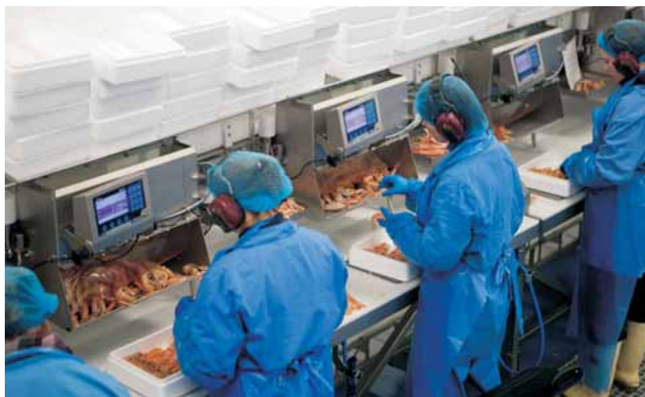
Each Marel weight grader is equipped with 24 ergonomically designed packing stations controlled by Marel Innova intelligent production management and monitoring software.
