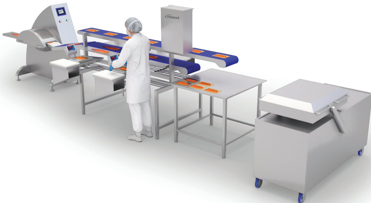
Slicing line with 1 single-lane slicer and a packing line for 4 operators.
