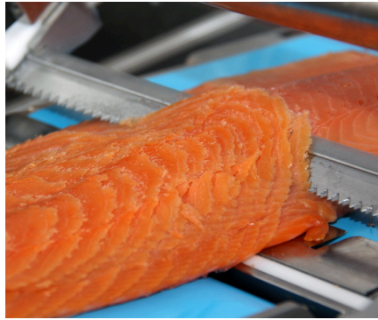
D-cut slicing: 18° – standard slices
