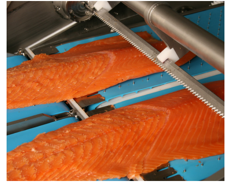
D-cut slicing: 10° – longer slices
