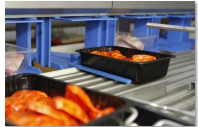
Tray Track consists of an overhead conveyor with tray carriers, automatic tray loading, unloading stations and electronic controls that are for programming and running the system
