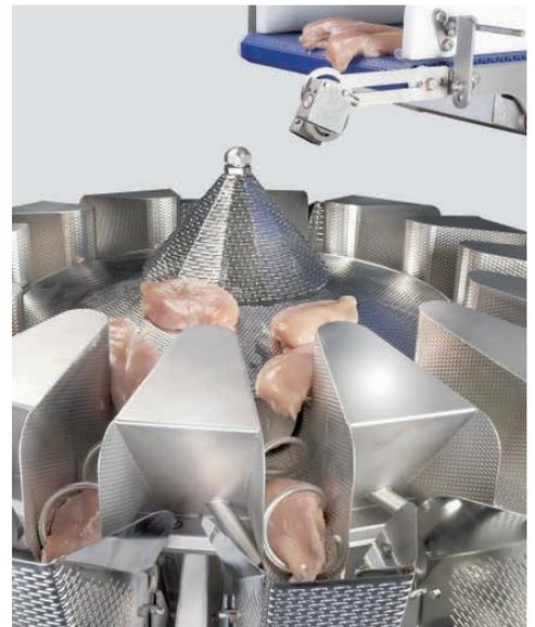
incoming product. Every time new products reach the weighing hoppers, the multihead weigher calculates all options for combining the available products and matches the results with the two target weights. The best option is then chosen. The batch will be created and released into the correct tray.
