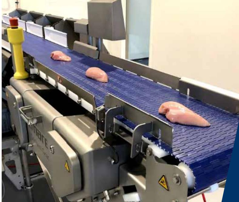
**“The Compact Grader has just one conveyor belt which needs cleaning. That’s all. Such short cleaning times of course add to the maximum uptime.”**
