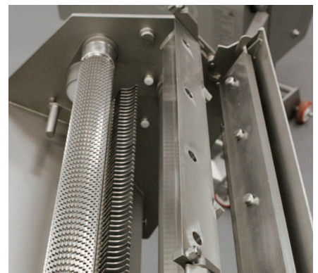
Easy to adjust air manifold for efficient cleaning and visual checks
