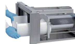
*Water tank removal at the top for all types of SAH 800 - 3000 and RVH 400 - 12000*
