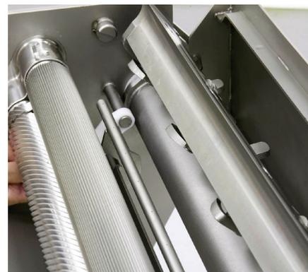
Easy to adjust air manifold for efficient cleaning and visual checks
