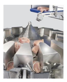
incoming product. Every time new products reach the weighing hoppers, the multihead weigher calculates all options for combining the available products and matches the results with the two target weights. The best option is then chosen. The batch will be created and released into the correct tray.
