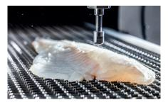
D3 water-jet robots move dynamically in all directions, giving maximum flexibility in portion shapes and sizes.
