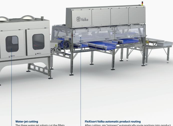
The three water-jet robots cut the fillets according to the specifications based on the X-ray and 3D scannning
