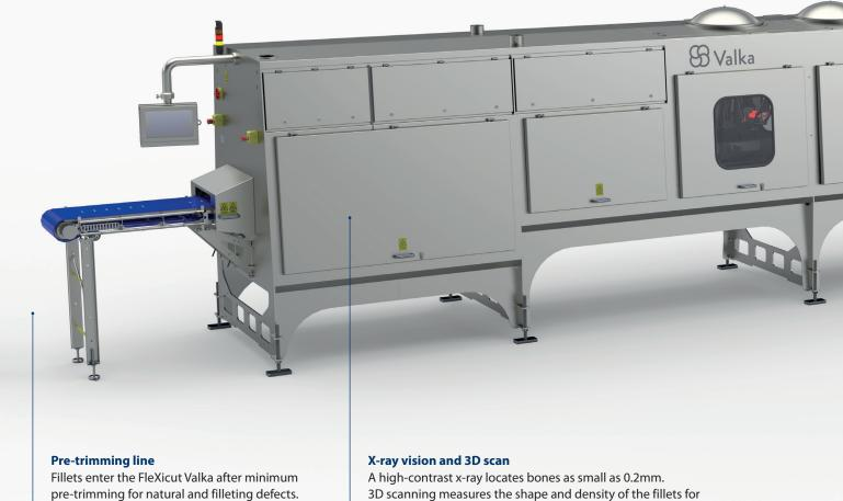
3D scanning measures the shape and density of the fillets for cutting based on weight.
