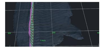
A 3D vision scan of individual fillets records, density, shape and size to ensure accurate portioning and prioritization of high-value cuts.
