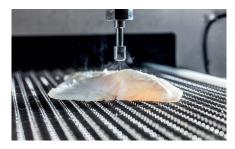
The robot tracking head assesses individual fillet height. Cut distances are adjusted to ensure the accuracy of endproduct quality
