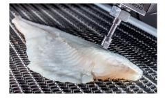
D2 water-jet robots move perpendicular to the fillet. By tilting to both sides, the D2 water-jet robots adjust angles to increase the proximity of cuts in pinbone removal.
