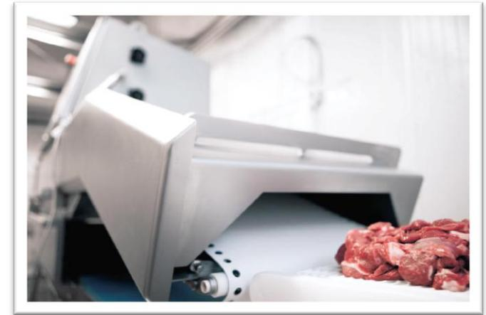
*Marel's new trim management system analyses the fat/lean ratio of meat using the X-ray technology of the SensorX, previously used so successfully to detect bones in poultry*
