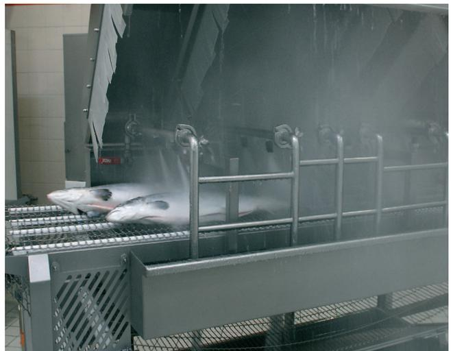
Efficient desliming with Marel Deslimer.
