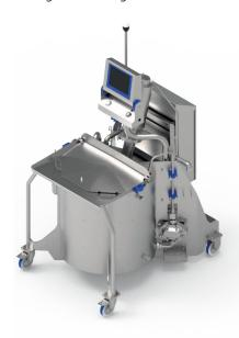
Correct mixing starts with the Active Mixer. After preparing a liquid mixture out of powder and water, the Active Mixer feeds this to a batter or tempura applicator. The system works intermittently, ensuring that the relevant applicator is filled in charges. A pressure pump can be used for heavier liquid mixtures, such as tempura.
