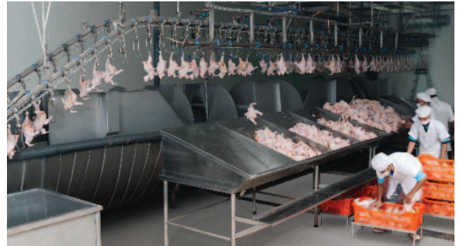
Distribution line with collecting bins for weight selection
