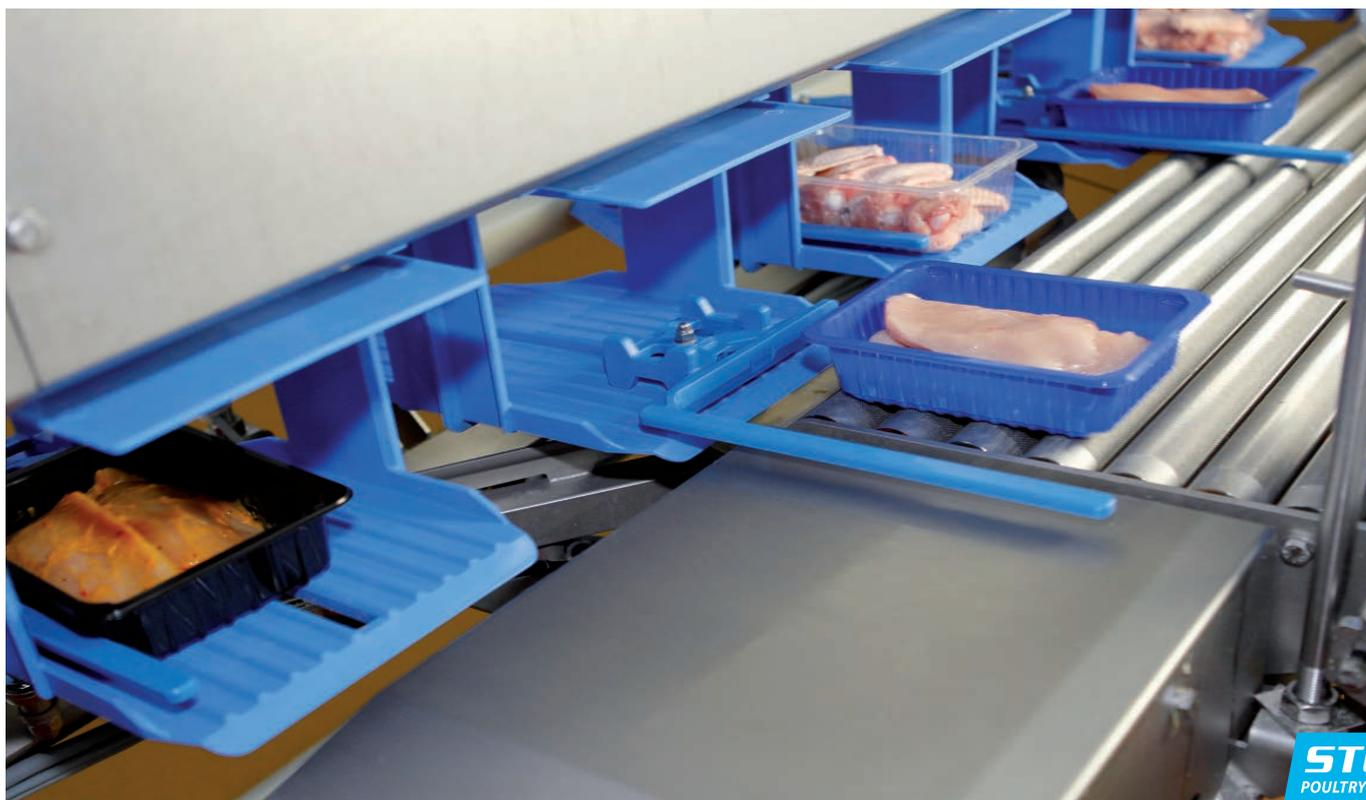
Trays are picked-up automatically at the loading station
