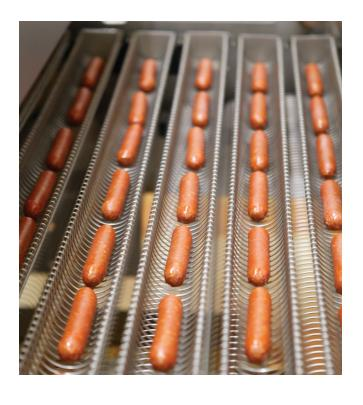
Traditionally, sausage are made by stuffing natural or preformed casings with meat dough. Another option is to create sausages using innovative co-extrusion technology. Here the casing is formed at the same time as the sausage is produced.
