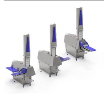
Three options for out-feed conveyer setup.
