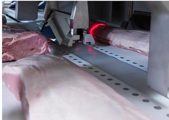
Product scanned by vision system for high-accuracy portioning.
