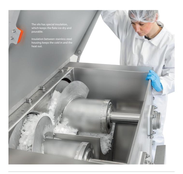
One or several MAJA flake ice machines automatically fill the IXT Silo from the top. The ice level indicator and ice production start time can be set via a user-friendly digital display to automatically refill the silo, keep ice levels optimal, and ensure fresh flake ice is available when needed.
