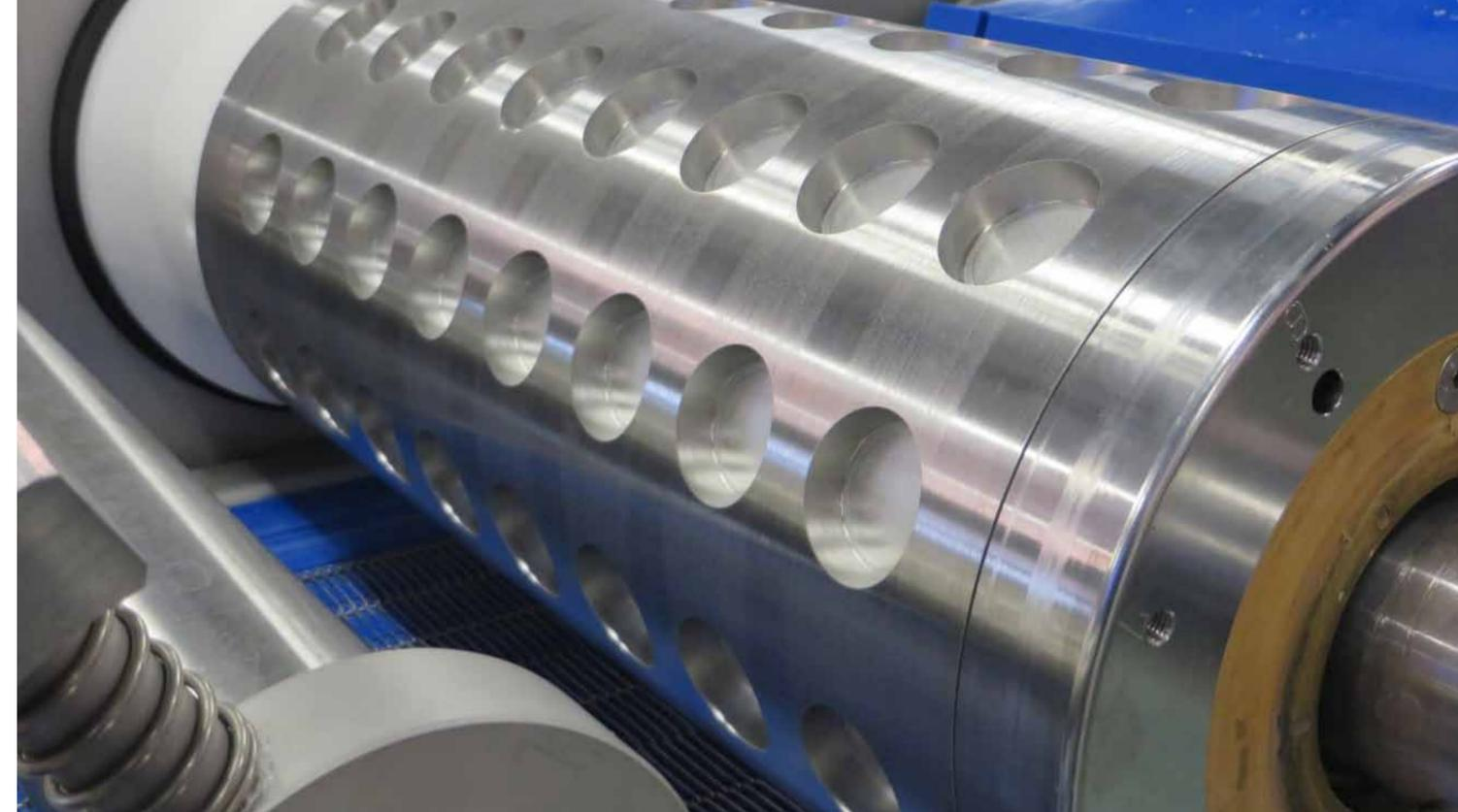
For test batches or development of new products, the New Product Development drum can be used. Its interchangeable segments allow you to experiment with different product shapes and sizes.
