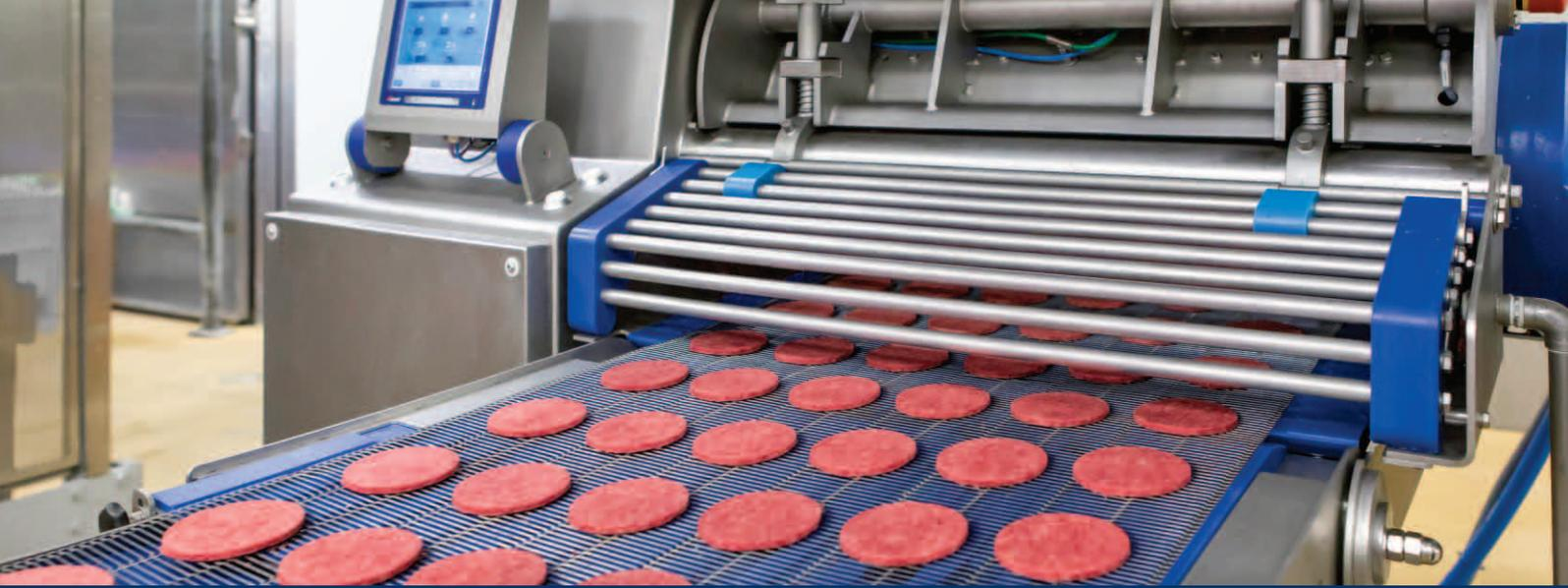
The V-Pump introduces a new high volume pump concept, producing up to 5,000 kilos of high quality convenience products on one system. Core of the new technology are two alternating belt-wide pistons, delivering a uniform pressure to the forming unit, moving the meat mass over a small distance with a minimum of pressure. This retains the original meat structure and texture as much as possible, an important factor for a good bite and attractive mouth feel.
