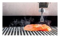
D3 water-jet robots move dynamically in all directions, giving maximum flexibility to portion patterns. They also move with the conveyor belt enabling larger fillets to be portioned.
