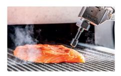
D2 water-jet robots move perpendicular to the fillet. By tilting to both sides, the D2 water-jet robots adjust angles to increase the proximity of cuts in trimming.
