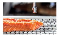
A robot tracking head assesses individual fillet height. Cut distances are adjusted to ensure the accuracy of end-product quality.
