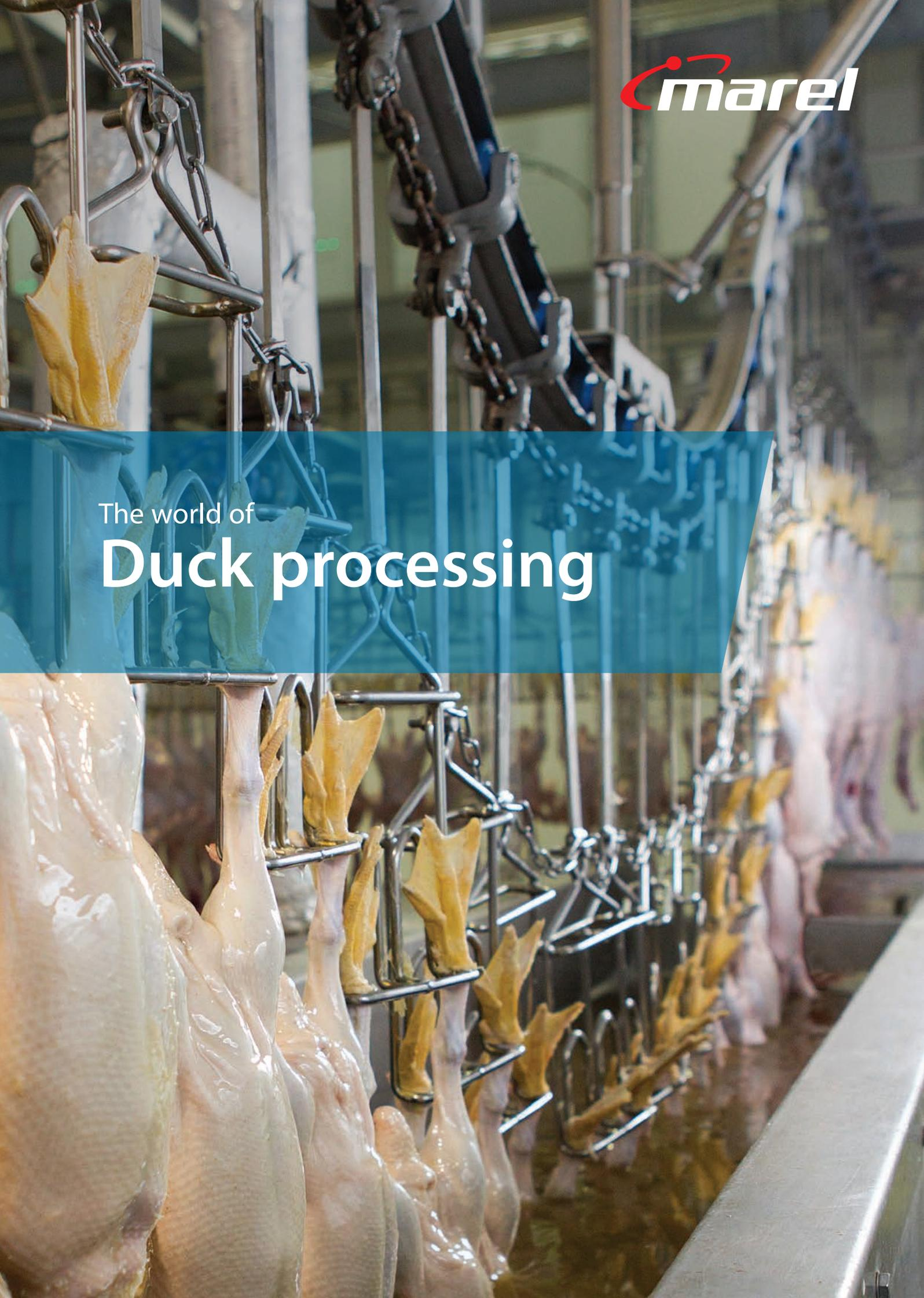
The background of the entire page is a photograph of a duck processing line. Ducks are suspended from a metal conveyor system. In the foreground, several ducks are shown with their legs tucked up, appearing to be in the scalding stage. The ducks are white and glistening. The machinery is made of stainless steel and includes various chains and rollers. The lighting is industrial and somewhat dim, focusing on the ducks.
