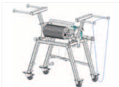
Pic. 1 Cleaning cart: With special fittings for comfortable cleaning of sanitizing-relevant machine parts, e.g. conveyer belts, pressure roller, knife holder etc.
