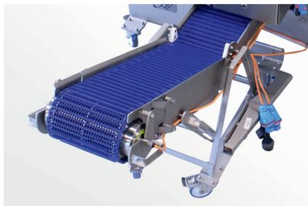
Unique takeaway conveyor to remove trimmings
